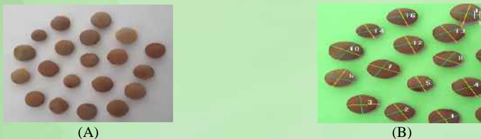
Figure 3. Examples of SmartGrain input and output. Scanned lentil seed for SmartGrain input (A). SmartGrain output highlighting segmented grains as determined by the software (B).
