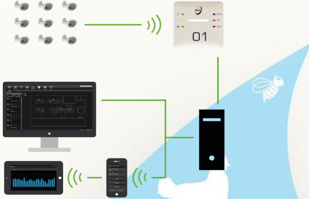
Figure 6. Example of RFID technology system with active ear tags and other components in barn
